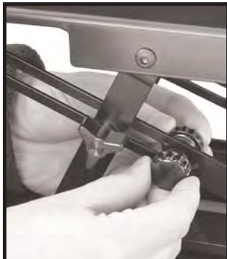
Assembly of plastic safety knobs - Do not remove them after installation.
